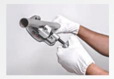
Cutting: Pipes are cut to length with approved burr-free cutters. Oxy acetylene torches and abrasive cut-off wheels are not suitable. Pipes are cut at right angles to their axis, using a pipe cutter or fine-tooth saw. Measured lengths must take into account the depth of insertion into the fitting.
