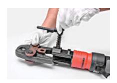
Press tool & jaw: Press tools are to be equipped with v-shaped profile jaw attachments or a pressing jaw which corresponds to the diameter of the fitting being pressed. Retract the lock pin, position the jaw in the tool head and fully engage the lock pin.
