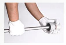
Deburring: Make sure that the internal and external tube end is free from burrs or sharp edges by using a deburring tool to prevent damage to the O-ring. Then wipe the tube end clean to avoid damaging the O-ring on tube insertion.
